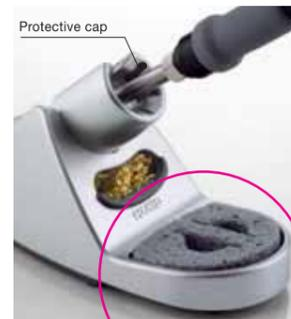
The corners on the iron holder base were rounded to prevent them from coming in contact with hand when storing the soldering iron. Further, a protective cap installed in the iron receptacle is provided to reduce sounds when storing the iron.
